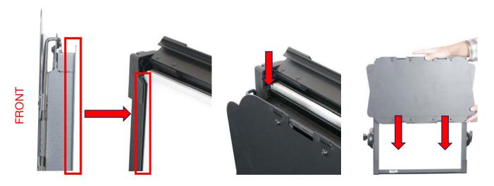
2. The inner frame of the fixture contains an empty mounting slot located just in front of the removable diffuser. Align the mounting rail on the rear of the barn door with this empty mounting slot, and slowly lower the barn door into place.
