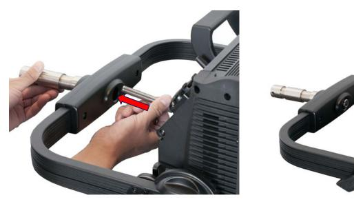
3. Thread the junior pin bolt in through the under side of the mounting yoke, making sure that the bolt engages the threaded hole in the junior pin. Tighten securely with a 10mm hex key. The junior pin is now ready for attachment to a clamp or stand.
