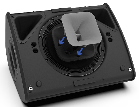
Grille removed, an additional magnetic flange can be quickly fitted to change directivity from 60°x60° to 90°x40°
