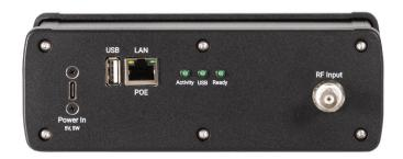
The RF Venue Spectrum Recorder, a compact and self-contained device, simplifies monitoring and optimizing wireless microphone and in-ear monitor systems. It continuously captures RF activity in the 400 – 700 MHz band, saving data as time-stamped CSV files on its internal storage. These files can be retrieved directly via USB drive or accessed remotely over a local network. Through its internal web server, the Spectrum Recorder can be operated over a network via GUI, with any web browser.
