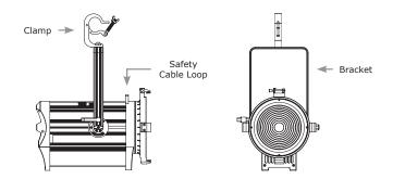
Mount the fixture using a suitable "C" or "O" type clamp. The clamp should be rated to hold at least 10x the fixture's weight to ensure structural stability. Do not mount to surfaces of unknown strength, and ensure properly rated rigging is used when mounting fixtures overhead.
